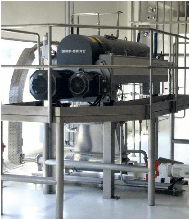
Decanter Model Z4E in soy milk production
