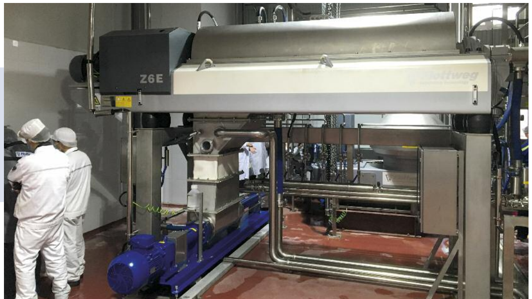
Decanter model Z6E used for the production of soy milk
